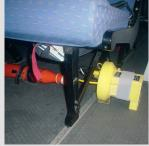
When your SAR mission faces adverse weather conditions, the safety equipment is used as a transponder sensitive to weather radar frequencies. Assisting in searching life rafts and helping the unit to point out exactly where the distressed boat is located, the ELT can also be removed from the aircraft to assist SAR teams in locating survivors of emergency.
