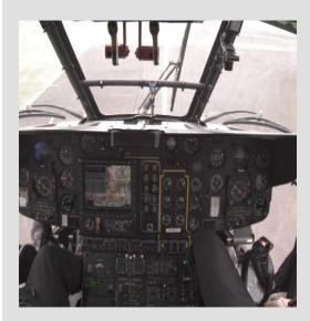
Vision 1000 is a low weight mini-Flight Data Recorder System installed in the cockpit. The system can record Attitude data, GPS, Cockpit imaging, and Ambient audio.
