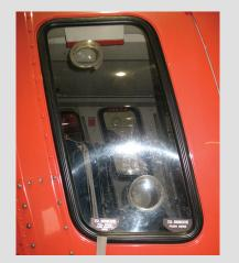
In the event of an emergency, exterior release straps installed on the exterior of the rotorcraft ensure quick pull out of these windows from the outside by rescuers.
