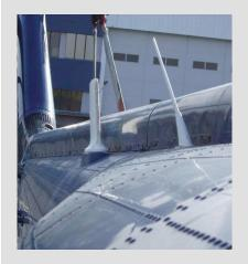
An upgrade to the S-61N for increased crew and passenger safety. Transmits the location of the helicopter in distress across multiple frequencies. Essential for operators working in remote and harsh environments.
