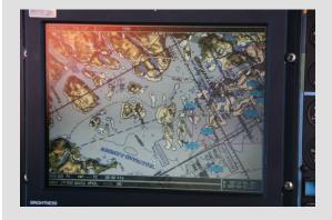
Improve your helicopter's marine navigation capabilities with this MFD installation, which includes the Euronav moving map system. An essential modification for those operating at sea.
