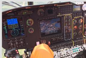
Heli-One offers a dual Flight Management System (FMS) upgrade for the Airbus AS332 platform. This upgrade uses the latest Satellite-Based Augmentation System (SBAS) technology, including GPS and LPV approach. The FMS includes a Multi-Mission Management System (MMMS) which allows the pilot to fly predefined patterns.
