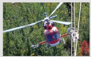
Versatile modification to the Airbus AS355 series which equips for specialist power line maintenance missions. The Deployment Boom can be flexibly used for a variety of purposes, including support of work stands, ballast and payload arms.
