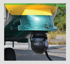
Axsys V9 is equipped with innovative infrared and HD daylight sensors to capture high-intensity target signatures day and night. Integrated with Aerocomputers UC-5100 tactical digital mapping system and rugged HD cockpit & cabin displays, the new system is an efficient, economical and powerful solution ideal for wide-area surveillance and remote monitoring missions.
