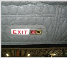
This kit replaces the typical hard interior trim with quilted blanket style lightweight items. All lights are replaced with low profile LED units.
