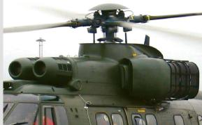
Provides enhanced safety while operating VFR and IFR in environments where shoulder-launched or other heat seeking missiles may be in hostile hands. Decreases the IR visibility of the aircraft with minimal consequence to performance.
