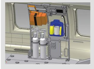
Placed in the aft part of the cabin, the Medical Equipment Rack is a removable rack that holds medical equipment used for SAR and Medevac operations.
