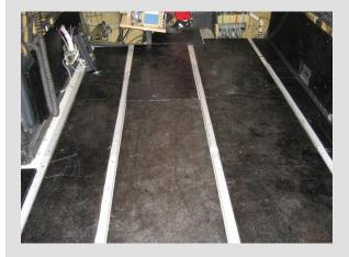
Maximizes protection for crew and passenger safety. Installed around existing equipment and access requirements, and enables interchangeability of armor panel units.
