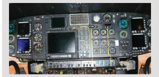
This EFIS (Electronic Flight Information System) display upgrade for Super Puma helicopters is designed as a cost-effective 'fully loaded' system with TCAS II, EGPWS/TAWS and GPS display capabilities as standard features.
