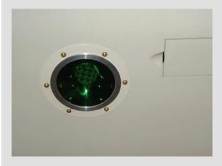
NVIS Dome Lights provides cabins with efficient lighting and the option to dim the lights from the flight deck.
