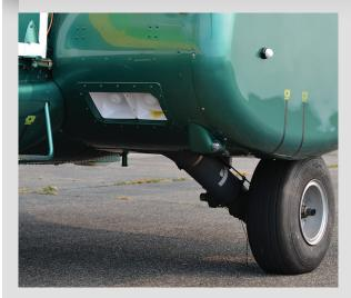
The Loud Hailer system is a public address system for communications between the flight crew and a person on the ground.
