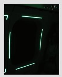
When operating offshore missions, make sure your aircraft is compliant with latest regulation by installing Helicopter Emergency Egress Lighting (HEEL). Designed to work even with the aircraft submerged, this modification helps passengers and crew find escape exits quickly in emergency situations.
